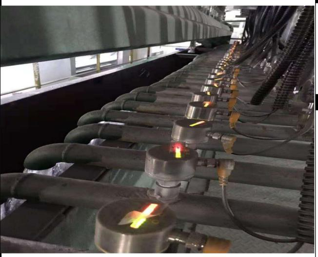
Because the previous brand often failed in the beginning, and also the price is increased. All flow sensors are installed on the cooling water pipes to monitor whether the cooling water stop flowing.
